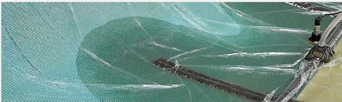
Example of a loading piece infusion with resin injection
